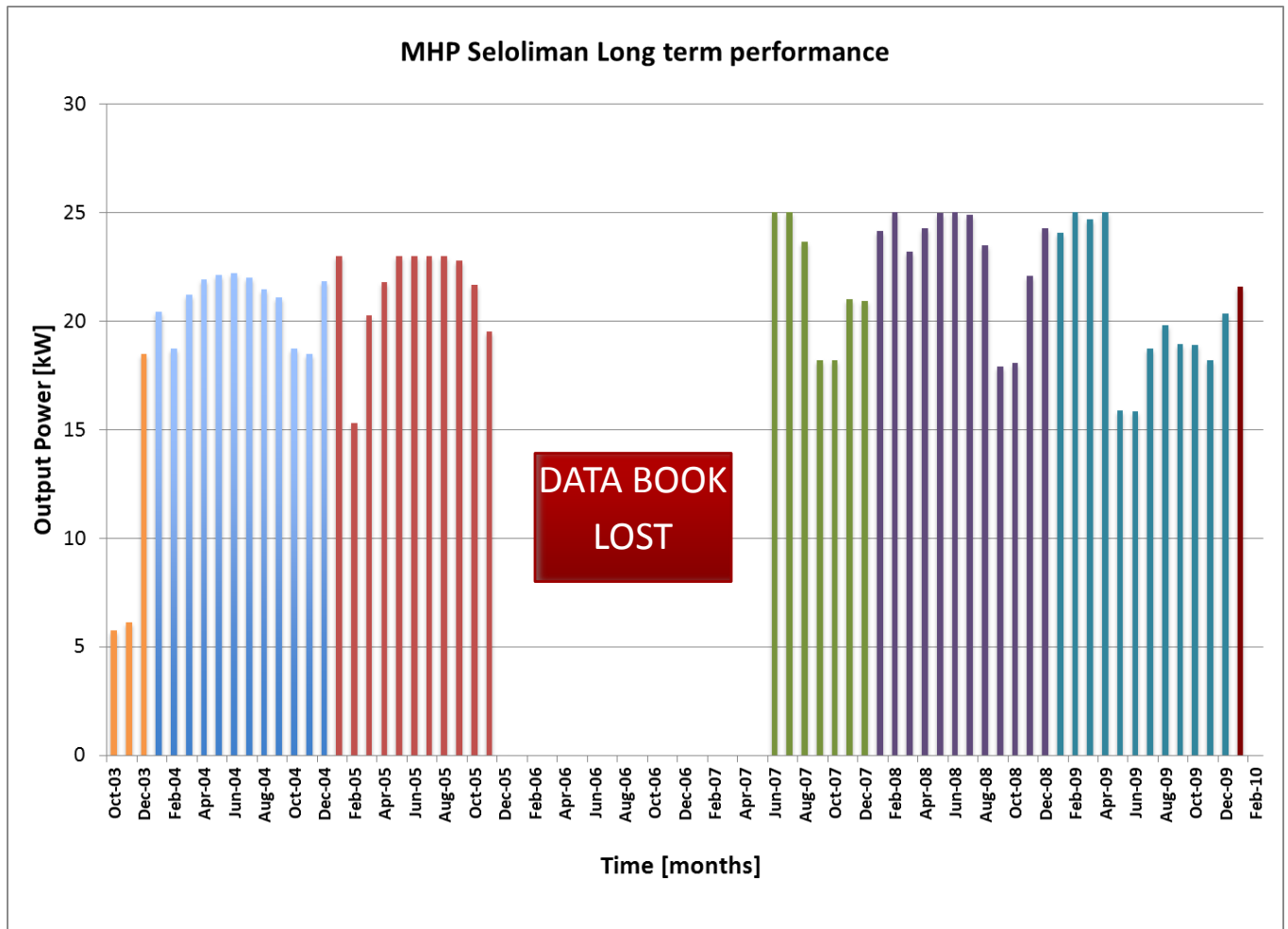
Graph 4.1. Seloliman Micro Hydro Plant long term performance. The output power values shown in the graph are an average of the monthly power output of the plant.
